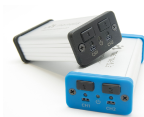
Figure 1. Electronic Control Units for monostable (blue cover) and bistable valves (black cover).
